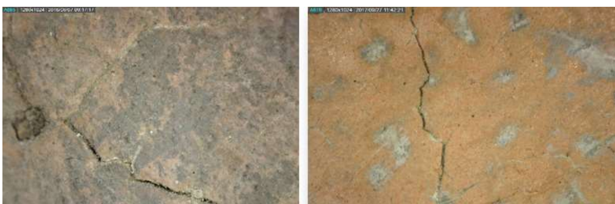
Figure 6. Example of microscope video documentation of the stone polychromy test area a) Before the cleaning treatment. b) After the cleaning treatment.
