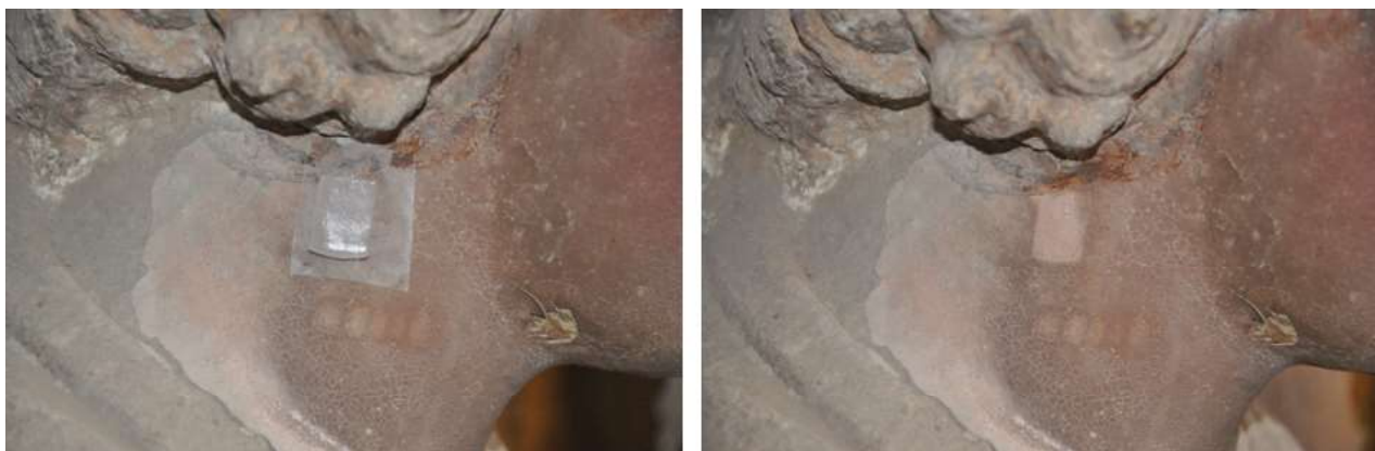
Figure 5. Application of the cleaning system with hydrogel in the test area in a polychrome figure of the Pórtico de la Gloria.
